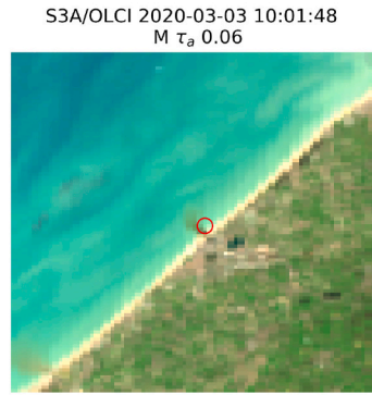
Fig. 5. A few selected matchups of Sentinel-3/OLCI and the PANTHYR deployed at RT1. The RGB composites use surface reflectances at 665, 560, 490 nm scaled from 0 to 0.15 in the 8 bit R, G, B channels. The open red circle on the RGB composites is centred on RT1. The title for each plot shows the aerosol optical thickness at 550 nm ( \tau_a ) and whether the Continental (C) or Maritime (M) aerosol model was used for ACOLITE/DSF processing. (For interpretation of the references to colour in this figure legend, the reader is referred to the web version of this article.)
