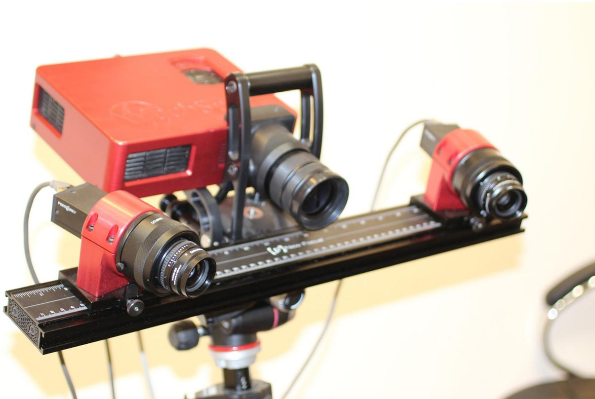
**Fig. 3.24.** The MechScan white light scanner.
