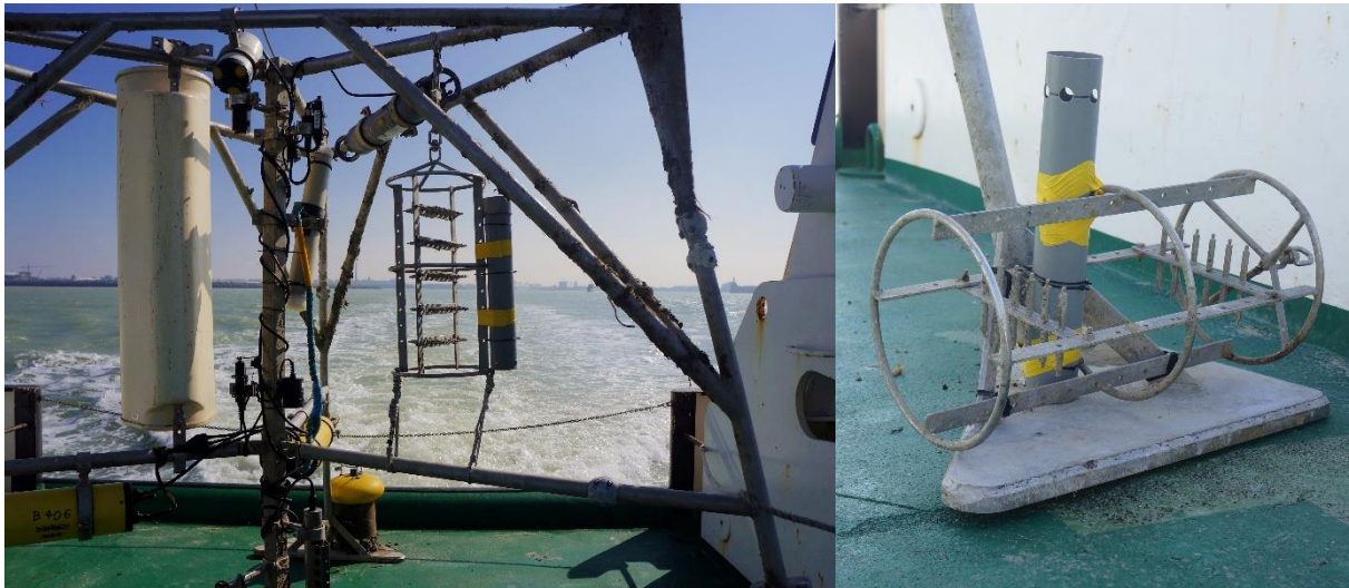
Figure 3.1: Tripod ready to be deployed at MOW1. Attached are left (white cylinder) the Technicap PPS4/3 and at the cage a CPIT (2mab). Right photo shows a 0.6mab PIT.
