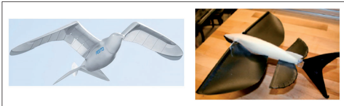
Figure 12. A flying robot inspired by the morphology and flying mechanism of herring gull 94 (Left); biomimetic marine robot inspired by Flying Fish. 95
