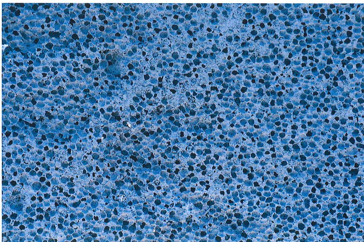
Lightweight foamed concrete is a substitute material for traditional concrete in building construction
