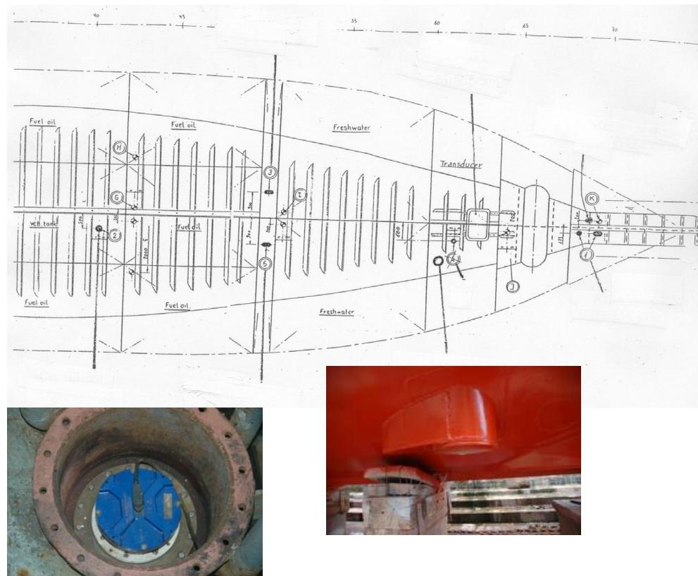
Figure 2.1: Location of the ADCP integrated in the hull of RV Belgica.
