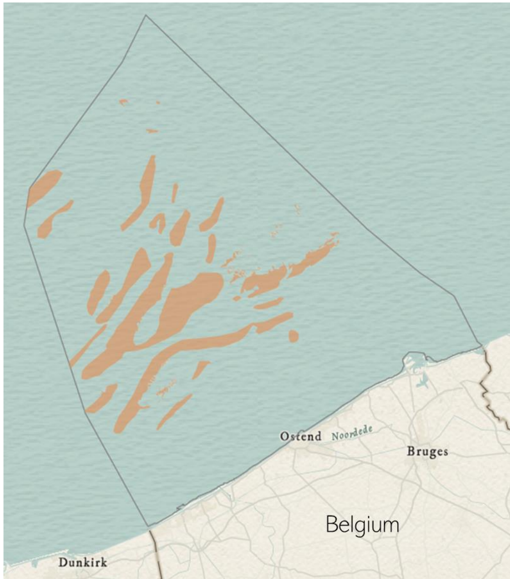
Figure 5. Spatial distribution of coarse sand and gravel potential occurrences (GIS@SEA dataset; Van Lancker et al. 2007, v2012) based on a combination of Quaternary sediment thickness maps, analyses of bathymetric data (single beam; multibeam where available), seabed samples (SediSURF@SEA dataset, Van Lancker 2007), and visual observations from video drop frames and diving information (mostly from the Belgian Navy). The gravel has varying sizes, contains shell material as well and may be buried under a sand layer. The map has been updated in 2009 and 2012 for nature management purpose. A complete revisiting is ongoing.
