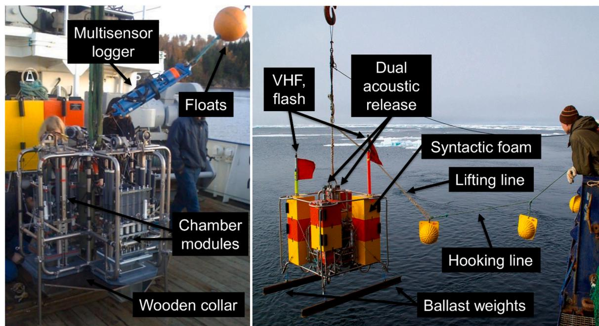
**Fig. 1.** Left: Inner frame of the big Gothenburg lander ready for deployment in shallow water with syringes and chambers armed. During deployment a multisensor logger is suspended above the incubation frame to record background information on currents, waves, salinity, temperature and oxygen. Right: Deployment of the big Gothenburg lander in autonomous mode with the outer carrier frame in the Arctic Ocean.
