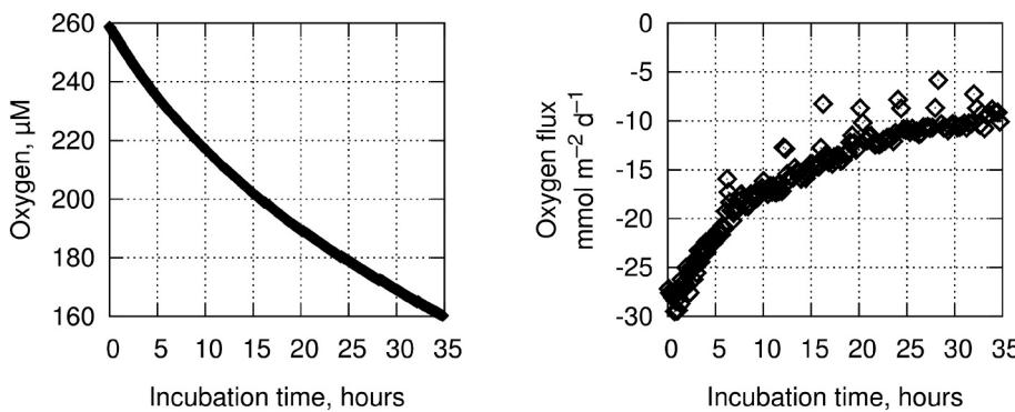
**Fig. 8.** Example from the northern Gulf of Bothnia at a water depth of 12 m of non-linear chamber oxygen dynamics in well oxygenated bottom water. In this extreme case oxygen uptake decreased from around 30 to 10  $\text{mmol m}^{-2} \text{d}^{-1}$ . Similar dynamics was also observed at deeper stations in the Gulf of Bothnia.
