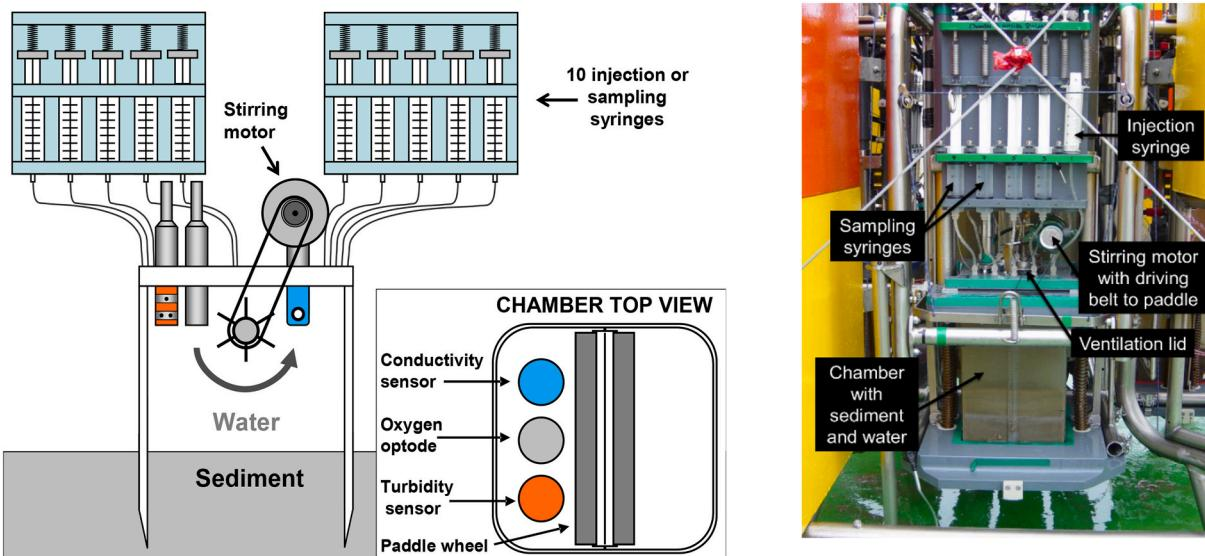
**Fig. 2.** Left: A drawing of the chambers used on the Gothenburg landers. Right: A photo of a chamber after big lander recovery with sediment and overlying water in the chamber, and syringes that have been triggered.
