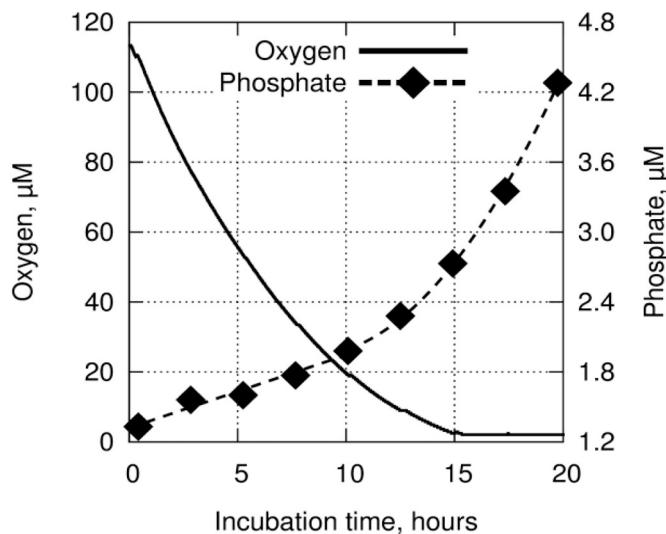
**Fig. 11.** Examples of the evolution of oxygen and phosphate concentrations versus time in a chamber of the big lander deployed in the deep part of the By Fjord. This lander deployment was made after the deep part of the By Fjord had been oxygenated by ecological engineering (Stigebrandt et al., 2015). Oxygen was measured at 1-min intervals with an optode. At a chamber oxygen concentration of about 20  $\mu\text{M}$ , the phosphate flux dramatically increased.
