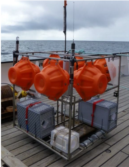
Figure A2. Photograph showing the baited free-fall lander trap designed and deployed by RBINS. Equipped with an acoustic release transponder, flashlight, Novotech radio beacon and Posidonia positioning signal to monitor position at the sea floor and ascension through the water column.
